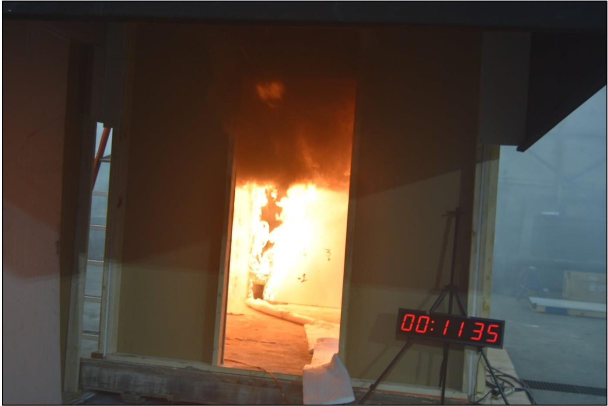
Figure A-7. Test at 11 min 35 s, Burner Output of 300 kW.
