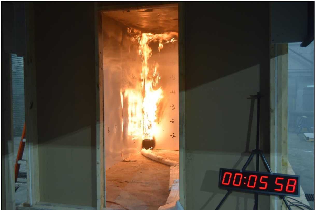
Figure A-4. Test at 5 min 58 s, Burner Output of 100 kW.
