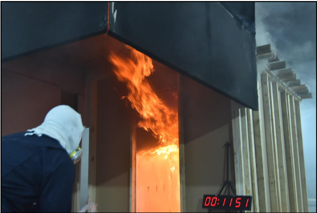
Figure A-8. Test at 11min 51 s, Burner Output of 300 kW. Flashover Conditions.
