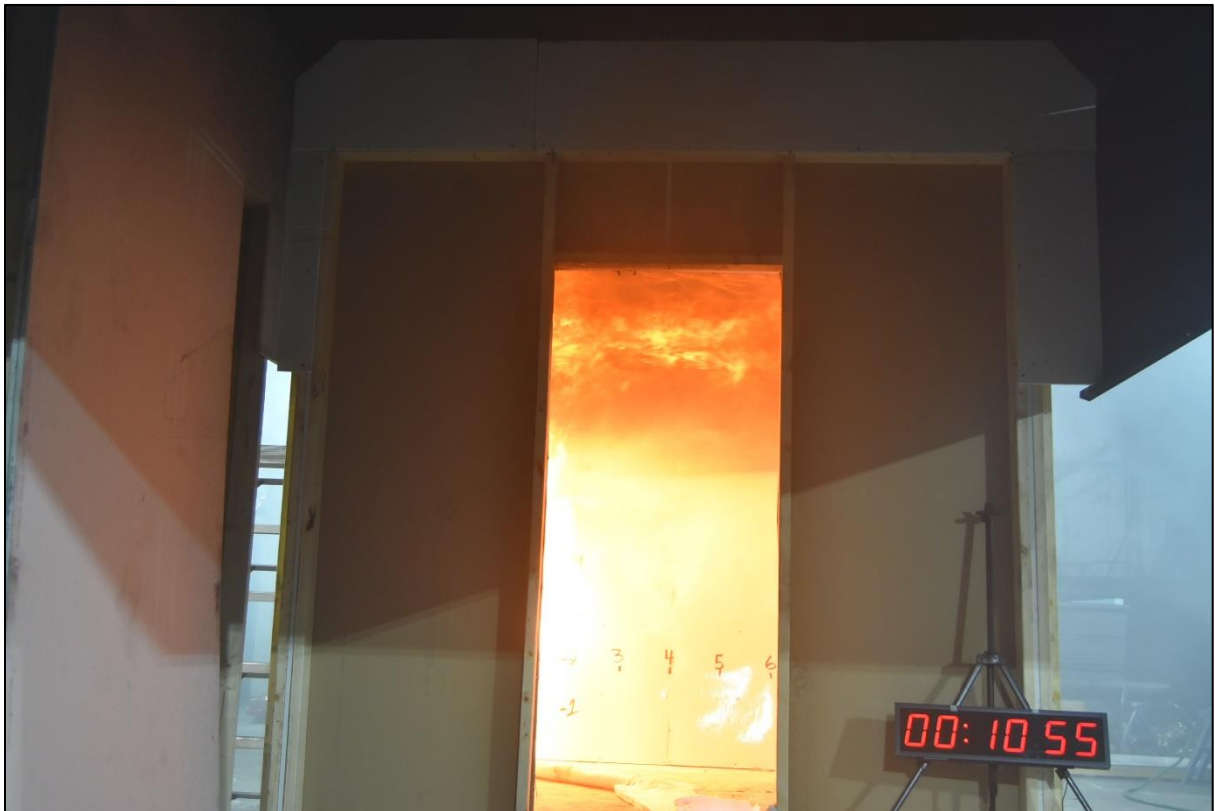
Figure A-6. Test at 10 min 55 s, Burner Output of 300 kW.
