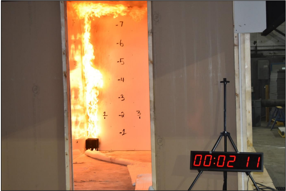
Figure A-3. Test at 2 min 11 s, Burner Output of 100 kW.
