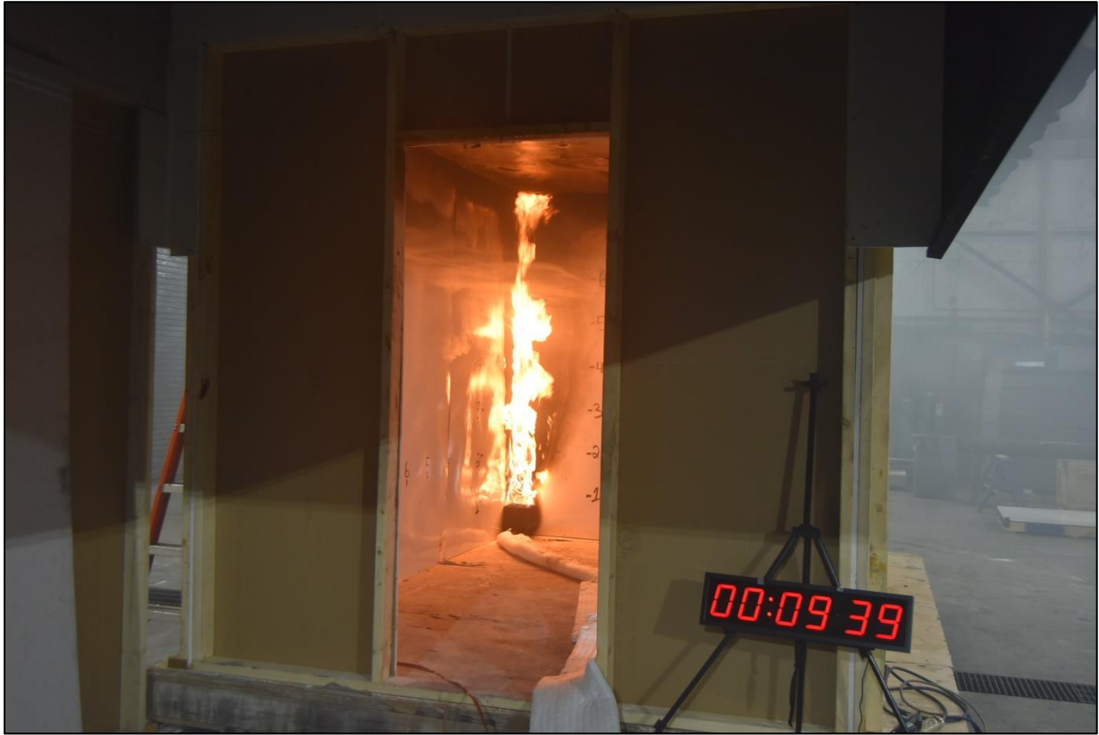
Figure A-5. Test at 9 min 39 s, Burner Output of 100 kW.
