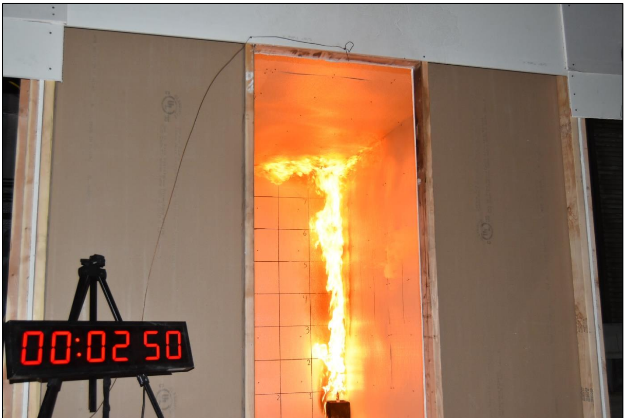
Figure A-4. Test at 2 min 50 s, Burner Output of 100 kW.
