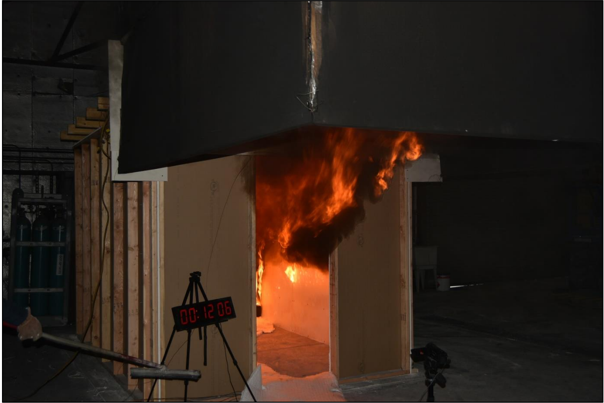
Figure A-9. Test at 12 min 6 s, Burner Output of 300 kW. Flashover Conditions.
