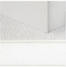
Foam substrates offer a lightweight panel construction that provides insulation and sound dampening properties. Foam cores are available in a number of different formulations (XPS, EPS, etc.) and densities depending on the performance required.
