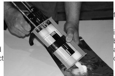
FIGURE 13: LEVELING THE PLUNGERS
