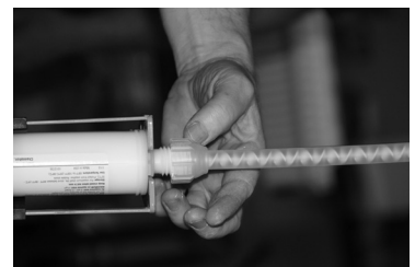
FIGURE 14: ATTACH STATIC MIXING TIP
