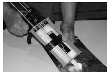
FIGURE 13: LEVELING THE PLUNGERS
